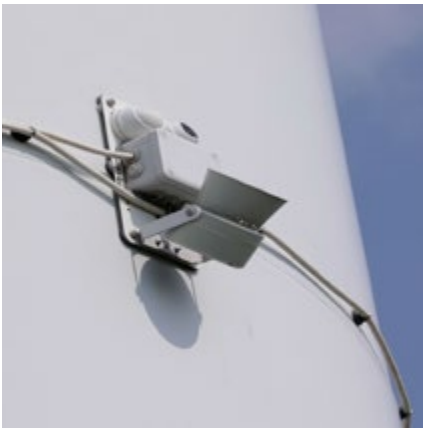
The SafeWind system (camera and horn) installed on a wind turbine
